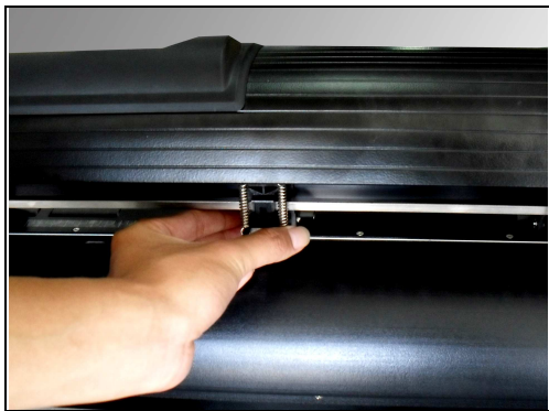
Figure 4-3 correct way to move pinch rollers
